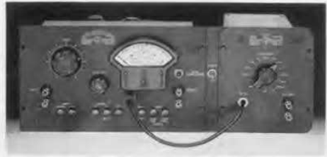
Figure 5. View of the Type 1231-PSR Filter arranged for relay-rack mounting with the Type 1231-B Amplifier and Null Detector. The filter panel attaches to the amplifier panel to make the assembly the correct width for mounting in a 19-inch relay rack. The narrow strip between the two panels carries a switch for the a-c power supply that is optional with the amplifier.
