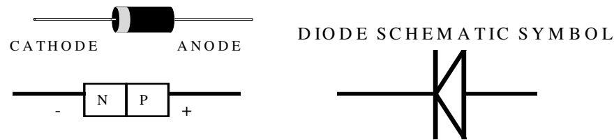
Figure 6-1. Diode and Schematic Symbol
