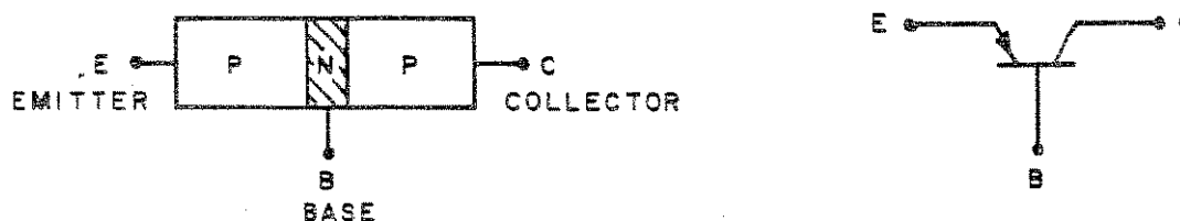
Figure 4-1. PNP Transistor and Circuit Symbol
