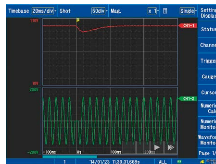
• Example of recording the instantaneous waveform and RMS level waveform during a momentary outage of an AC power supply (using the MR8905)
