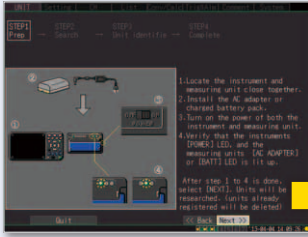
QUICK SET easy setup screen (shown when the Wireless Logging Station is turned on)
