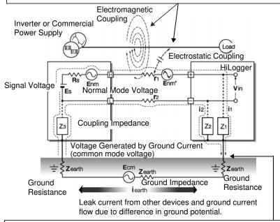
Common mode noise results from the interposition of ground impedance between the ground point of the device being tested and the ground point of the HiLogger, and from capacitor coupling between the ground wire and noise source.
