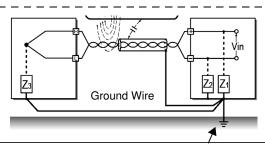
If the signal side is not grounded or if it is grounded inadequately, connect the HiLogger to ground. Also ground the shielding for the signal wires on the HiLogger side securely.
