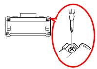
4 Align the connectors on the HiLogger and the input unit, mate them together, and secure with the attached screws.
