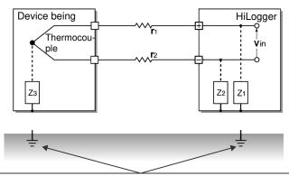
When using a thermocouple to measure temperature, noise can affect measurements unless both the device being tested and the HiLogger are grounded.
