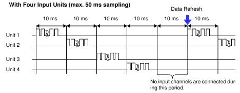
When the digital filter is off, the scan widths and dead times between channels are fixed to the values shown in the figure above regardless of the recording intervals. When the digital filter is on, the scan widths and dead times between channels vary in accordance with the recording intervals.
