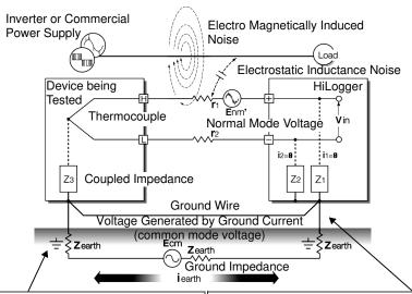
Connect the chassis GND on the signal side to a good ground with a sufficiently low ground resistance. If there is still a large amount of noise, it may be possible to reduce the effects of common mode voltage by connecting a bypass ground wire to the GND terminal on the HiLogger.
