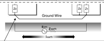
If it is not possible to simply ground the HiLogger or the signal side, connect a ground wire between the chassis GND of the HiLogger and the signal side to equalize ground potentials. A basic requirement for obtaining stable measurements is to ground the device.
