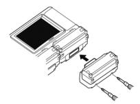
Mount the extension input unit on the side of the HiLogger with the metal hooks, and tighten the screws securely.
