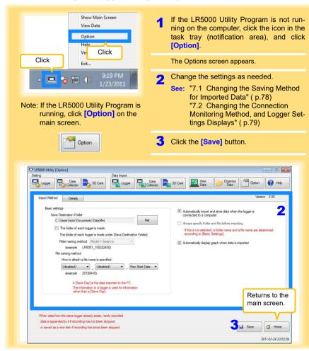
Select the [Automatically import and store data when the logger is connected to a computer] checkbox and clear the [Always specify folder and file before importing] check box to display the Data Import screen (p.55).
