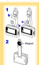
1 Attach the Z5004 to the strap/stand attachment hole.
