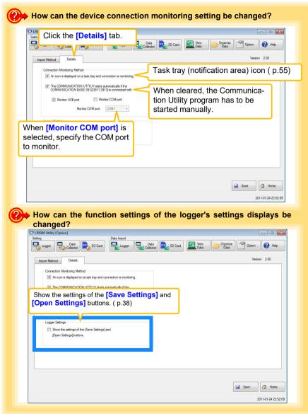
7.2 Changing the Connection Monitoring Method, and Logger Settings Displays
