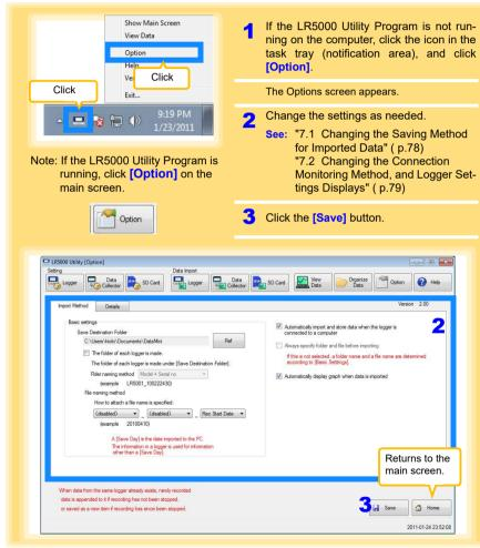
Select the [Automatically import and store data when the logger is connected to a computer] checkbox and then clear and the [Always specify folder and file before importing] check box to display the Data Import screen (p.56).
