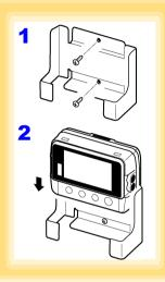
Mount the LR9901 to the wall using the two screws.
