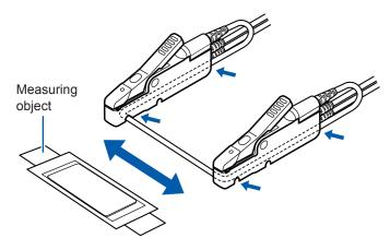
If the measurement is difficult, fixing can be done at the center. However, effectiveness of noise cancellation will reduce. (The return cable is indicated black in the illustration.)
