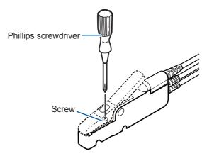
2 Adjust the stopper position by moving the stopper back and forth and tighten the screw.
