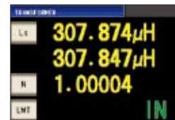
Transformer measurement mode Turn ratio measurement and judgment screen
