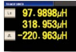
Transformer measurement mode Inductance difference measurement screen
