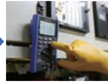
Press the MEM key to save measured values in the instrument's internal memory.
