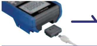
Optical communications link
