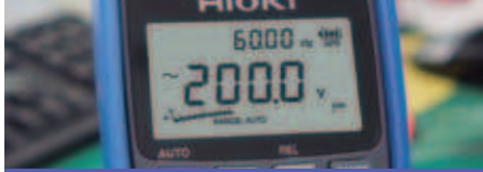
Dual-value and bar graph displays
