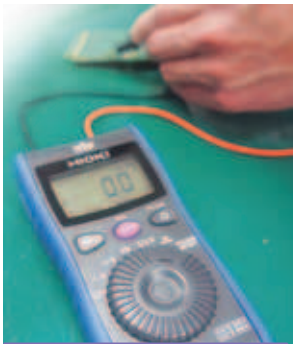
Test leads plug into the rear
