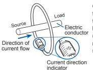
Clamp only the conductor you wish to measure with the current direction indicator pointing toward the load side.
