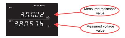
In the  $\Omega$  mode, the measured resistance value appears on the upper display.
