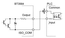
PLC Input (Source Input) Connections
