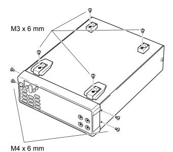
1. Remove the feed from the bottom of the instrument, and the screws from the sides (four near the front).
