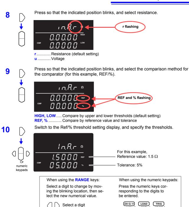
To enter the current measured value: AUTO key (Press on a screen other than the upper/lower threshold setting display.) To enter the result of statistical calculation value: STAT key (Press on a screen other than the upper/lower threshold setting display.) See " Upper and Lower Thresholds Setting (by Reference Value and Tolerance)" (⇒ p.52).
