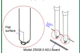
The sense side of the tip of the test lead has a flat surface. When using the zero-adjust feature, orient the test lead so that the surface the same direction.
