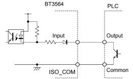
PLC Output (Sink Output) Connections
