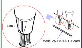
Each sensor pin has a line affixed to its base. When using the zero-adjust feature, orient the test lead so that the surface the same direction.
