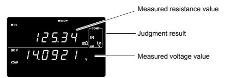
In the  $\Omega V$  mode, you can verify comparator settings by pressing the **VIEW** key. See " Switching Between Measurement Value and Comparator Setting Displays" (⇒ p.56).
