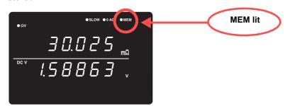
If an external trigger source is selected, one measurement is stored after each trigger event. In the internal triggering case, the first measurement value after triggering is stored. Apply a trigger as many times as is necessary.
