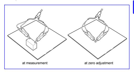
These variations are particularly pronounced in the 3 m $\Omega$  and 30 m $\Omega$  ranges, so be sure to position the leads in same state as will be used to perform actual measurement when using those configurations.
