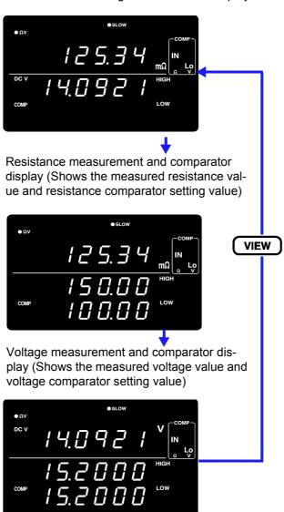
Measurement display switching is available only with the comparator enabled, and in the  $\Omega V$  mode.
