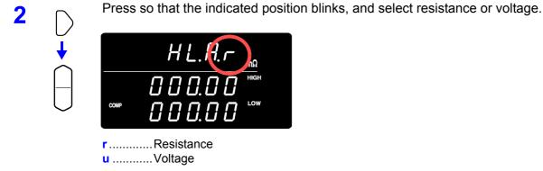
Select the threshold setting display, and enter upper and lower threshold values.
