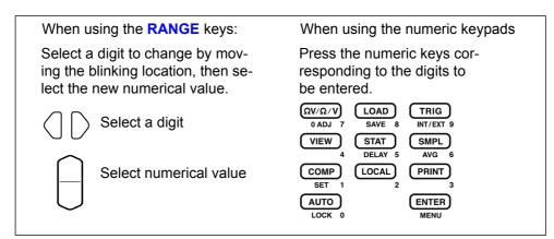
To enter the current measurement as the setting value: AUTO key Press on a screen other than the upper/lower threshold (reference value/tolerance) setting display. This key is used as a numeric key on the upper/lower threshold (reference value/tolerance) setting display.
