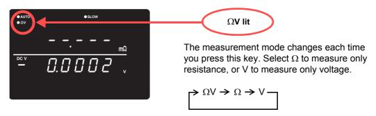
Set the measurement range. (for this example, 30 m $\Omega$  range is selected.) See "3.4 Setting Measurement Range" (⇒ p.27).
