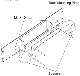
2. Installing the spacers on both sides of the instrument, affix the Rack Mounting Plate with the M4 x 10 mm screws.
