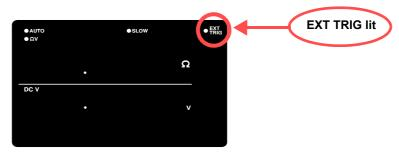
**EXT.TRIG** lit...... External triggering is selected. **EXT.TRIG** not lit....... Internal triggering is selected.
