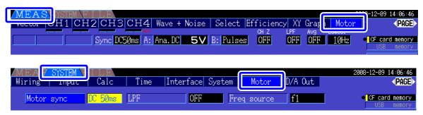
The motor analysis function acquires signals from rotation-sensing devices such as a torque sensor and rotary encoder and measures motor analysis items (torque, rotation rate, motor power and slip). Motor efficiency, total efficiency and loss can be calculated when combined with the 4.7 Viewing Efficiency and Loss Measurement Values (p. 78) functions.
