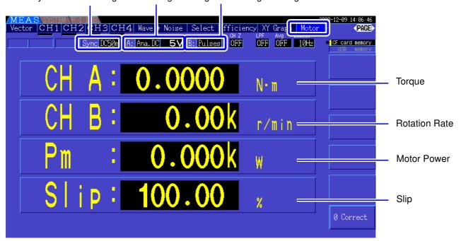
See Motor measurements can be displayed simultaneously with motor input voltage and current, power measurements and motor efficiency. "Selecting Measured Items for Display" (p. 38)
