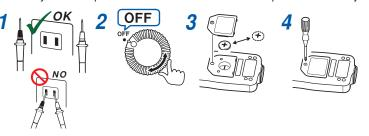
Do not turn the adjustment screw inside the battery case. Doing so will cause the instrument to report abnormal measured values.
