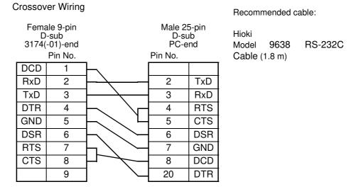
Note that the combination of a dual male 25-pin D-sub cable and a 9- to 25-pin adapter cannot be used.
