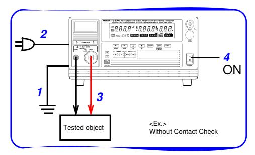
"Connecting the Protective Conductor Terminal" (p. 18)
