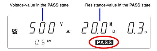
In the initial setting, **PASS** will light up for about 0.3 seconds before returning to READY mode.
