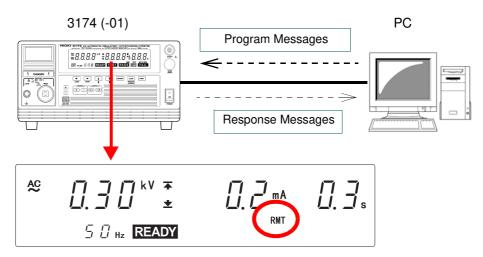
**"RMT**" lights up on the screen during communication, the instrument switch to the remote state.
