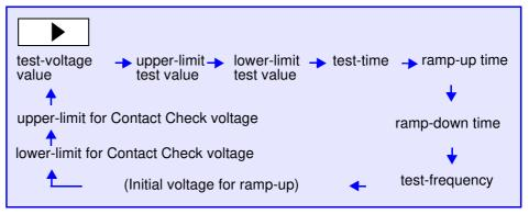
If the item is not needed in the test, set it to OFF using the **ON/OFF** key. However, the test-voltage value, the upper-limit test value, and the test-frequency cannot be set to OFF.
