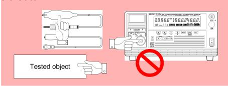
When a test object that contains a capacity component is subjected to a test, the object might remain electrically charged, thereby causing an electric shock.
