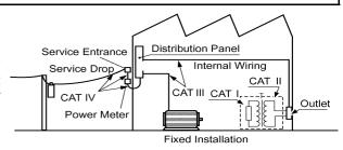
Using a measurement instrument in an environment designated with a highernumbered category than that for which the instrument is rated could result in a severe accident, and must be carefully avoided.
