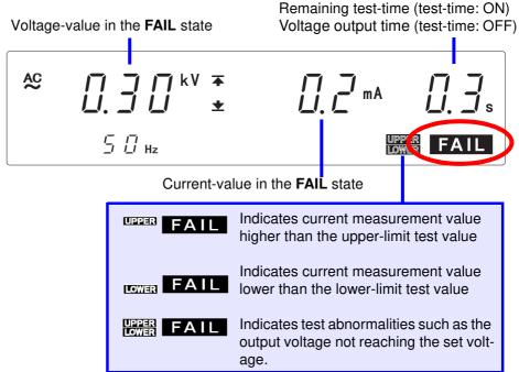
To return to the READY state, press the **STOP** key, which will cancel the FAIL Hold function.
