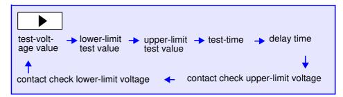
If the item is not needed in the test, set it to OFF using the **ON/OFF** key. However, the test-voltage value and the lower-limit test value cannot be set to OFF. Pre-set test conditions can be saved.
