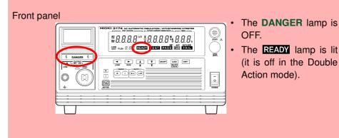
The test result is displayed on the screen. "PASS" or "FAIL" screening is conducted according to the insulation-resistance test termination mode settings based on whether a measured-resistance value exceeded the upper- or lower-limit value.
