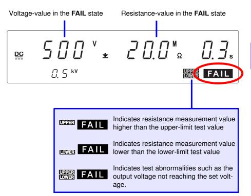
When the FAIL status is retained, to return to the READY state, press the **STOP** key, which will cancel the FAIL Hold function. In normal tests, the time from when the instrument achieves and detects a FAIL evaluation to the time when the output voltage becomes OFF depends on the size of the capacity property of the tested object.
