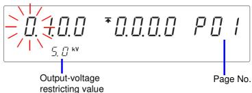
Press the key to move the flashing cursor to the position of required function.
