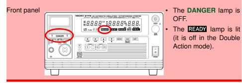
The test result is displayed on the screen. "PASS" or "FAIL" screening is conducted based on whether a measured-current value exceeds the upper- or lower-limit test value within the set test-time.
