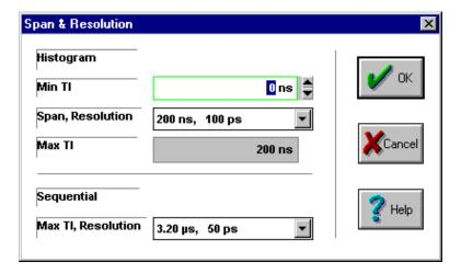
This window configures the fast histogram hardware to cover the range of intervals being measured. Since this drive has a decode window or "T" spacing of 15.6 ns and uses RLL (1,7) coding, intervals will cover the range from 2T to 8T (31.2 ns nominal to 124.8 ns nominal). A span of 200 ns is chosen to cover this measurement range for the histogram. The resulting histogram bin width, or resolution, is 100 ps.
