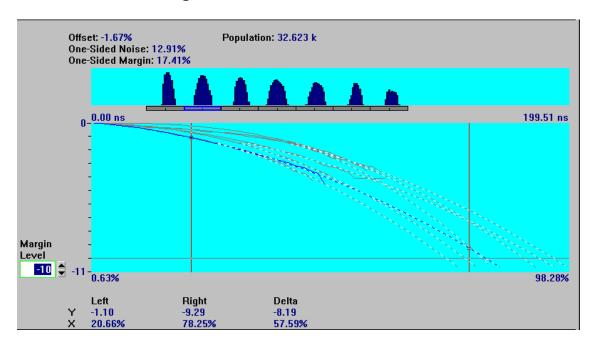
This display shows the one-sided window margin plot, with the segments overlaid. The one-side margin plot is computed by "folding" all of the distributions about the segment centers, adding the selected segments together, and computing window margin from this single-sided histogram.
