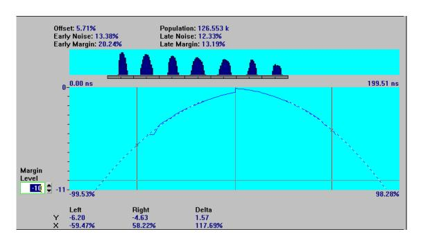
This display shows window margin computed from the histogram, using the segment definitions created earlier. The panorama display shows the original histogram distributions, and the main display shows the computed two-sided window margin. The dashed line is the extrapolated curve through  $10^{-10}$  margin level.
