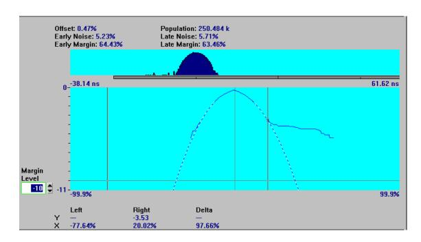
Notice that the new late window curve fit ignores the break-away in the window margin data and more closely approximates the rest of the acquired data in the window margin curve. The resulting margin is much closer to the early window margin.
