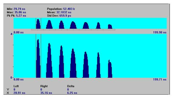
This histogram result display clearly shows the seven time interval distributions corresponding to the 2T through 8T code spacings. The upper display is called the panorama display and always shows a full view of all the data acquired. You can "zoom-in" or magnify the data by pressing the ↑ key on the keyboard. The larger, main display will show the magnified view.
