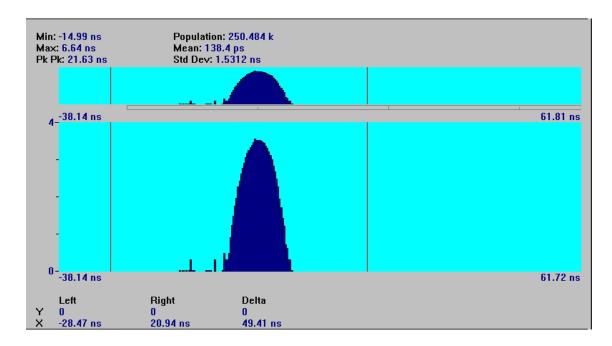
This histogram display shows a single histogram distribution, corresponding to the data-to-clock measurement configuration. With dual-channel measurements there are often systematic timing differences (skew) between the measured edges of each channel. This can occur for numerous reasons: cable length differences, propagation delays in circuit access points, etc. The TIA has been calibrated so that internal path length differences should not contribute significant timing skew.
