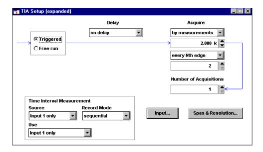
Review the setup menu for the frequency settling measurement. The HP E1741A is triggered with a voltage step and will gather 2,000 measurements, timing every second data edge. Notice also that the "Record Mode" is set to "sequential." The HP E1741A will record timing information in its 512K sequential memory, as opposed to processing data into histograms on-the-fly as shown in the earlier demos.
