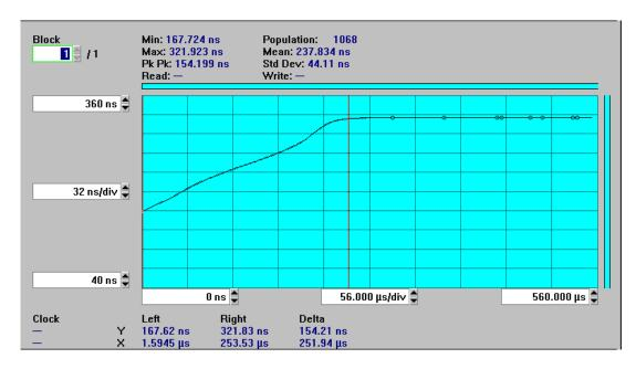
This is the HP E1741A's "measurement" vs. time display of sequential, or continuous, measurement data. In this example, the display is "time interval vs. time." The markers work much the same as for the histogram display, as you can click on either one with the mouse and drag it to the desired location. Statistical values are presented at the top of the display for the data between the current position of the markers. Marker values and differences are displayed at the bottom of the display.
