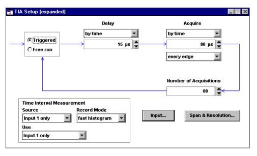
This is the TIA setup menu to make data-to-data measurements on the drive under test. The screen is configured as a flow diagram showing the various stages of the measurement. Reading from left-to-right you can see that the TIA will wait for a trigger, delay 15  $\mu s$  and then measure every edge for 80  $\mu s$ . This sequence is repeated 80 times, which results in the acquisition of 80 consecutive sectors.
