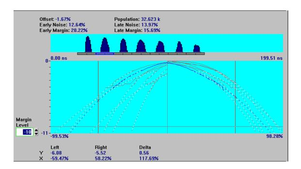
This display now shows the window margin curves for the individual distributions overlaid, rather than combined. One segment beneath the histogram is highlighted (in blue). Its corresponding window margin curve is also highlighted in blue on the main display. The window margin results and the marker readouts correspond to this selected segment.
