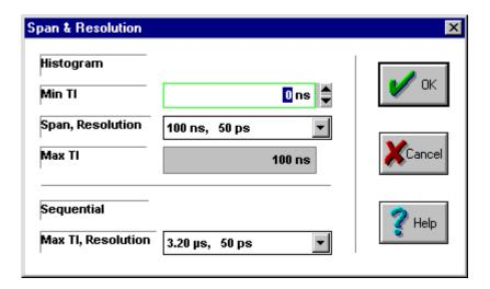
A dialog box is opened. There are two parts to this form, Histogram and Sequential. The upper part sets the boundaries for the histogram, the lower sets the boundaries for sequential measurements.
