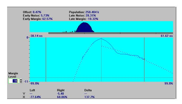
These are the corresponding window margin results for the data-to-clock histogram. Due to the incorrect delay from trigger value, the histogram (shown above the window margin) has a number of measured intervals that are set apart from the main distribution. You can see these on the left side of the histogram on the panorama display.
