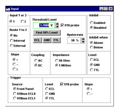
This screen configures the input circuitry on the HP E1725C TIA for the particular signals from the drive under test. The data signal (connected to input 1) has a 50% point at 3.7 volts, and a X10 probe is connected to the test point. Hysteresis, or sensitivity, is set to 50%.
