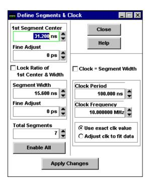
This window allows you to define the number and position of the segments and define the clock. Since this drive has a 15.6 ns decode window, the first distribution (2T) is located at 31.2 ns. The RLL (1,7) coding dictates that there should be 7 segments. These segment definitions are also used for window margin calculations. Since data-to-data intervals are used for display and analysis for this demonstration (instead of data-to-clock), the clock definition is not required.
