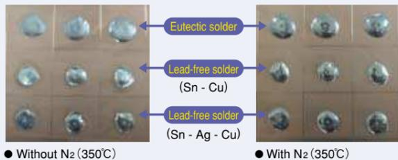
Less bridge is generated even for components susceptible to bridging.
