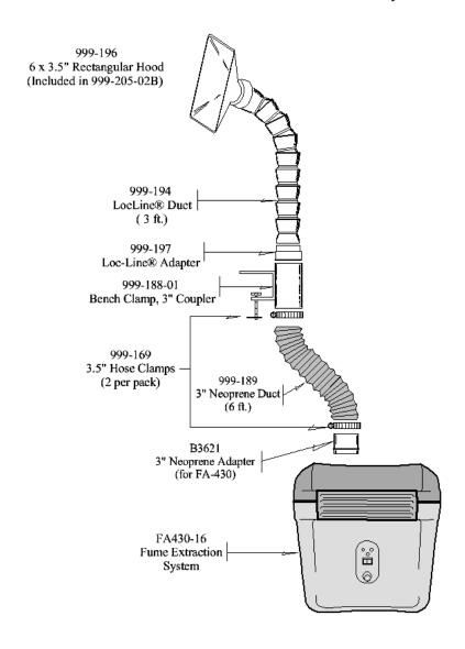
NOTE: Ensure the Neoprene Duct is attached to the longer side of the Neoprene Duct Adapter as measured from the flange.
