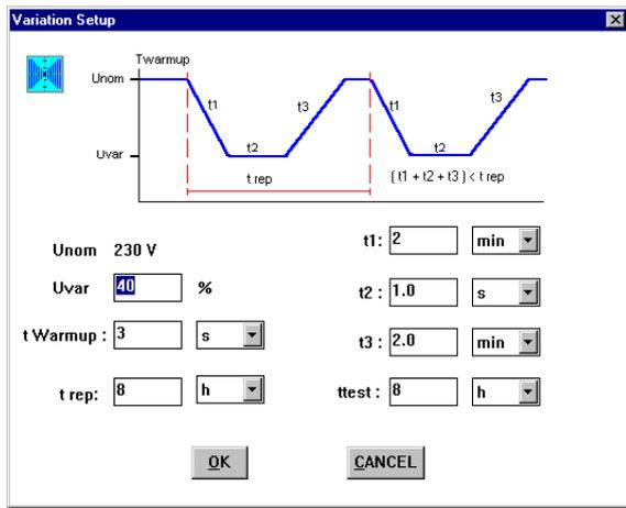
WinFEAT&R software used to control the PLINE 1610, means that magnetic field testing can be automated with other EMC tests.
