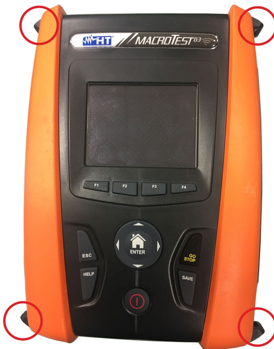
Fig. 42: Instrument with fitted half-shells and hooks
