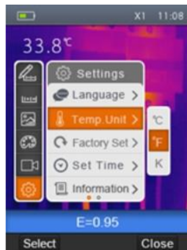
Fig. 9: Setting the temperature measuring unit
