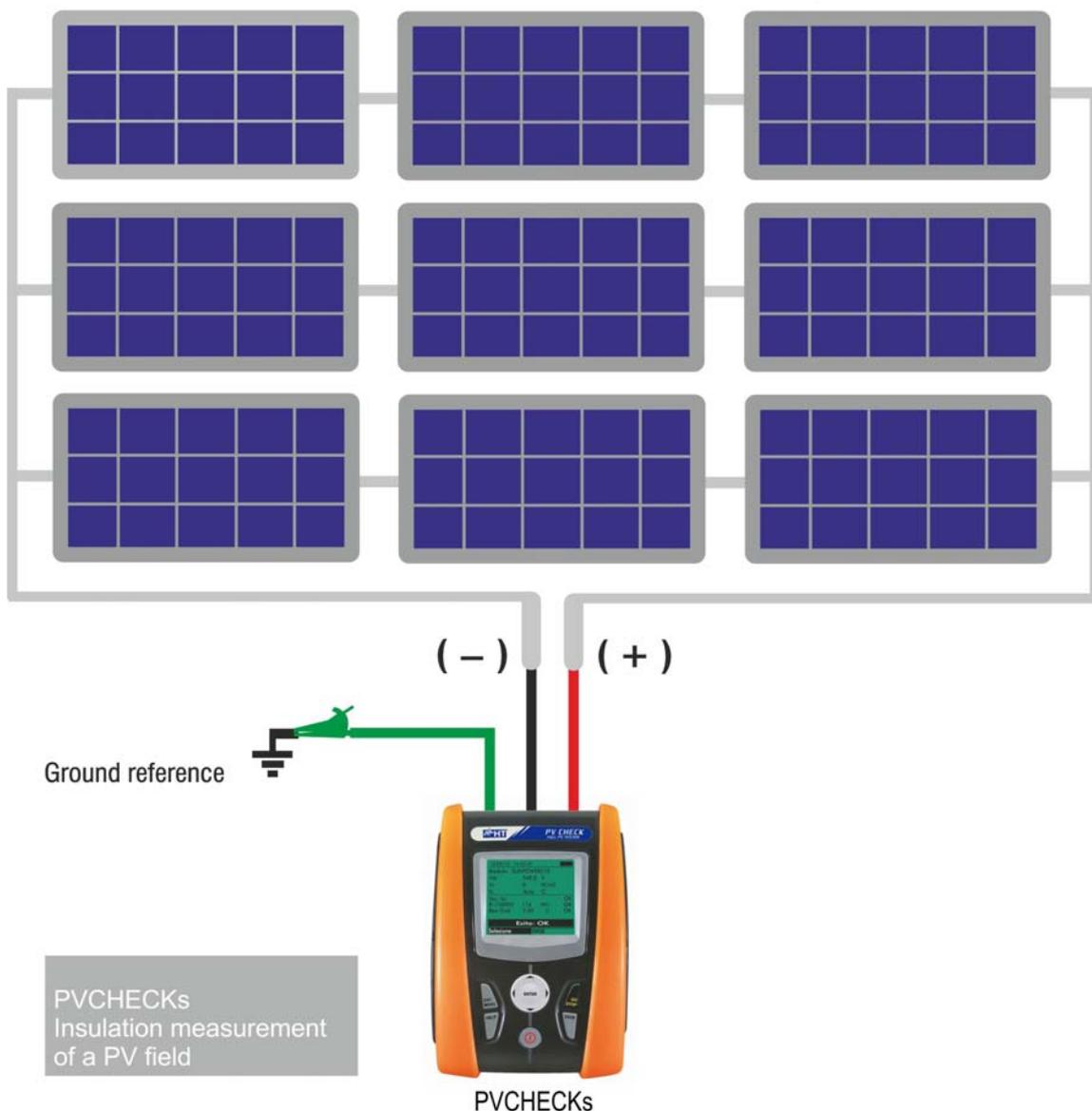
Direct measurement of insulation resistance of a PV Field not connected to ground
