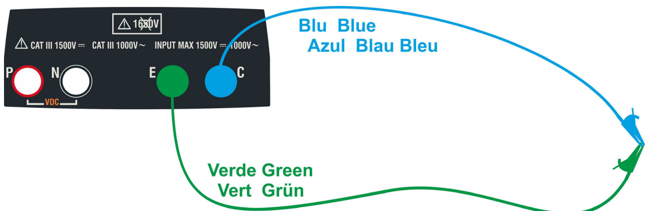
Fig. 4: Compensation of the measuring cables resistance
