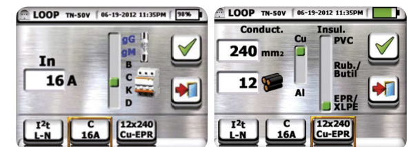
Setting of MCB/fuse type and rated current
