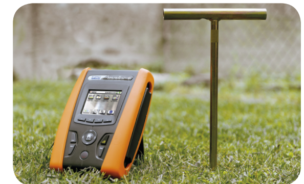
Earth resistance measurement by Volt-ampere method
