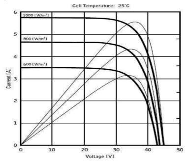
On each characteristic curve there is one single point in which the power transfer towards a hypothetical charge supplied by the photovoltaic module is maximized. The maximum power point corresponds to the voltage-current pair for which the product V\*I is maximum, where V is the value of voltage at the module's terminals and I is the current which runs in the circuit obtained by closing the module on a hypothetical charge.
