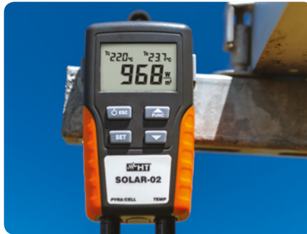
Solar02 remote unit.
