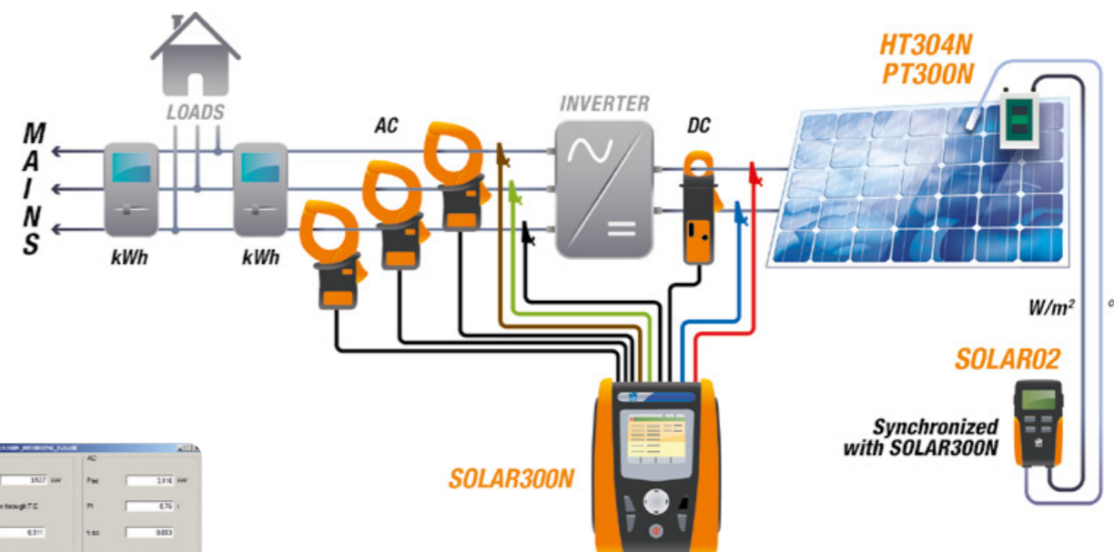
Connection diagram (three-phase system)
