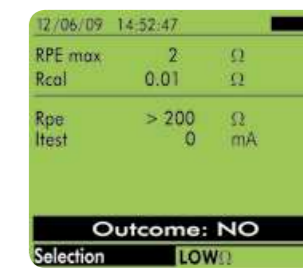
Continuity test result with 200mA NOT OK
