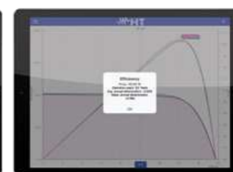
Comparison between foreseen cell deterioration and measured value.
