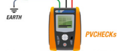
Insulation measurement with method "whole photovoltaic field"
