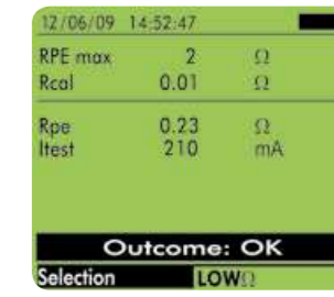
Continuity test result with 200mA OK
