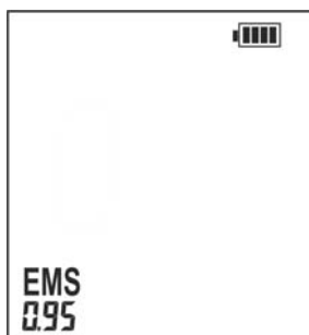
Fig. 8: Setting the emissivity value of the surface
