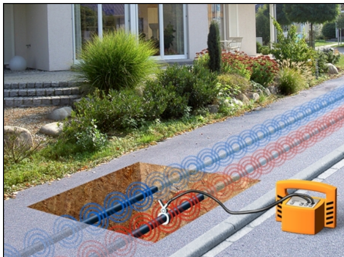
Fig. 6: Coupling via transmitter clamp
