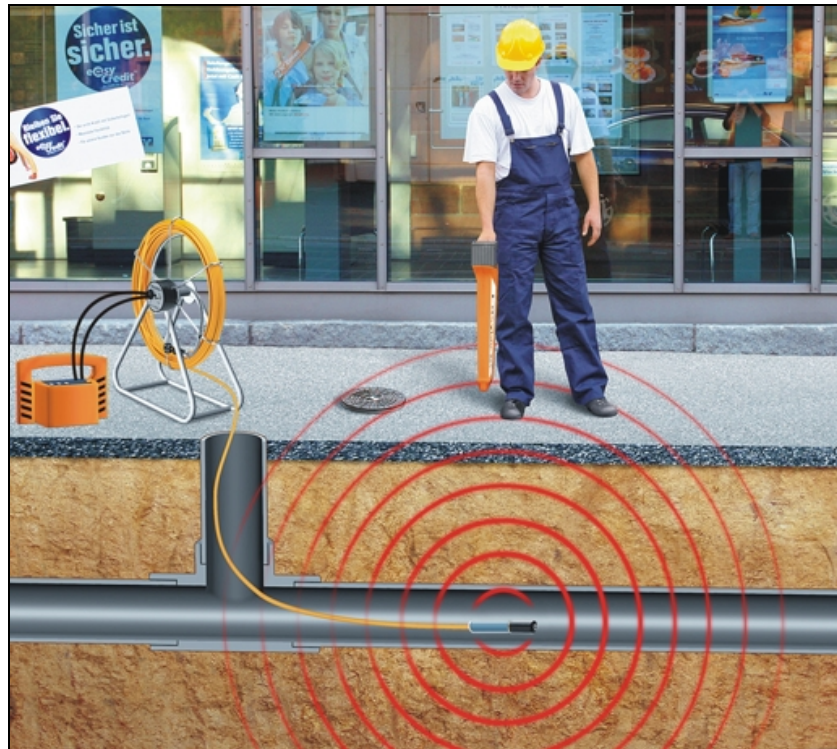
Fig. 9: Signal coupling in non-metallic pipes
