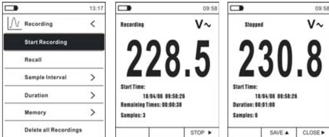
Fig. 37: Data logger function – Starting and stopping recording
