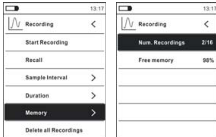
Fig. 41: Data logger function – Content of the memory
