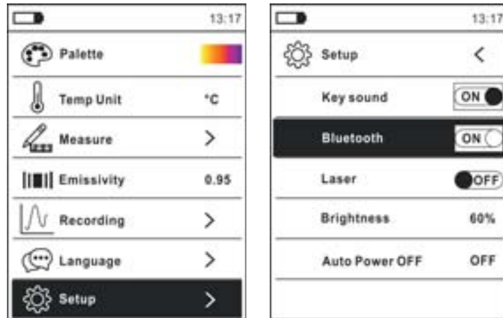
Fig. 47: Activation of Bluetooth connection
