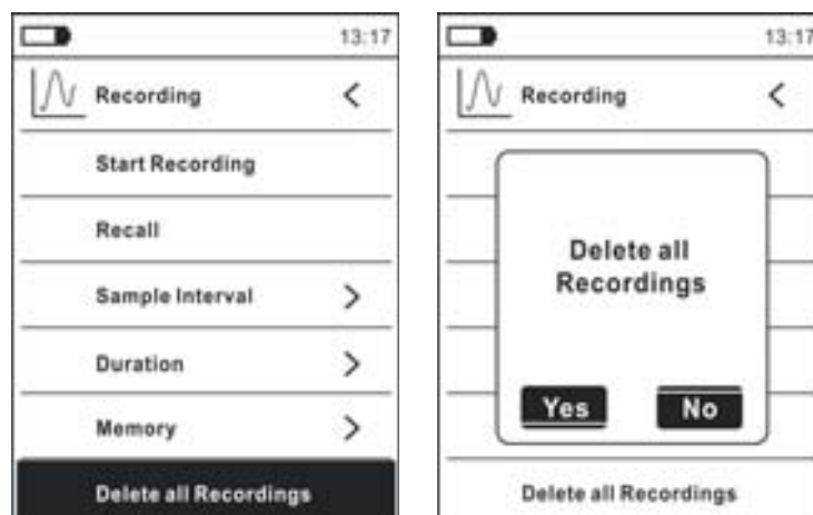
Fig. 42: Data logger function – Deleting all recordings
