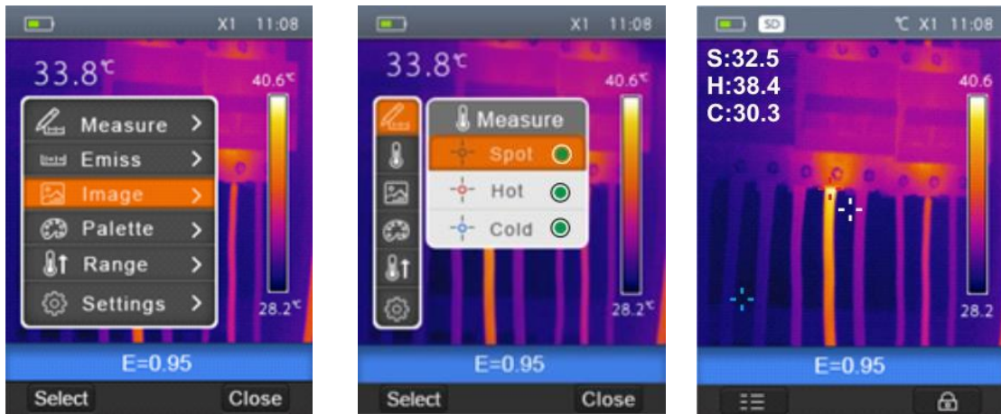
Fig. 17: Setting of measuring cursors
