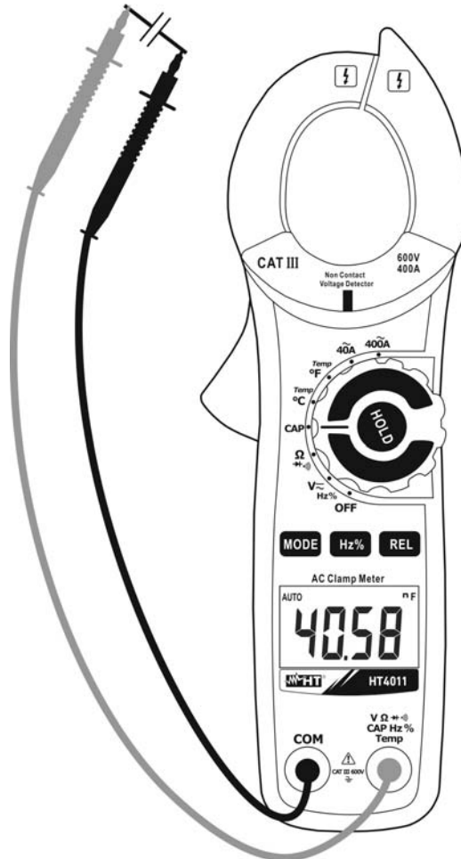
Fig. 6: Use of the clamp for capacitance measurement
