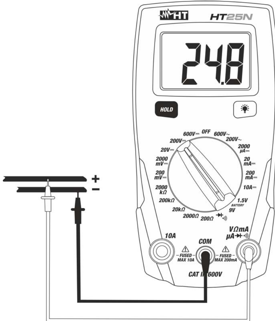
Fig. 2: Using the meter for DC Voltage measurement
