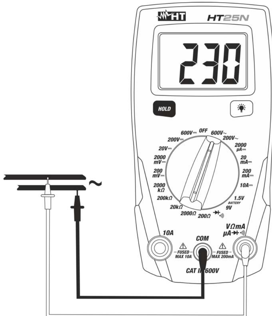
Fig. 3: Using the instrument for AC Voltage measurement
