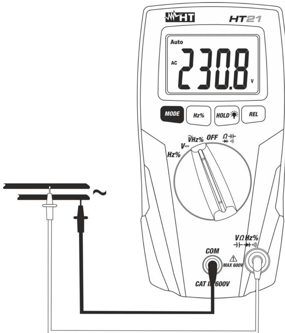
Fig. 3: Using the instrument for AC Voltage measurement
