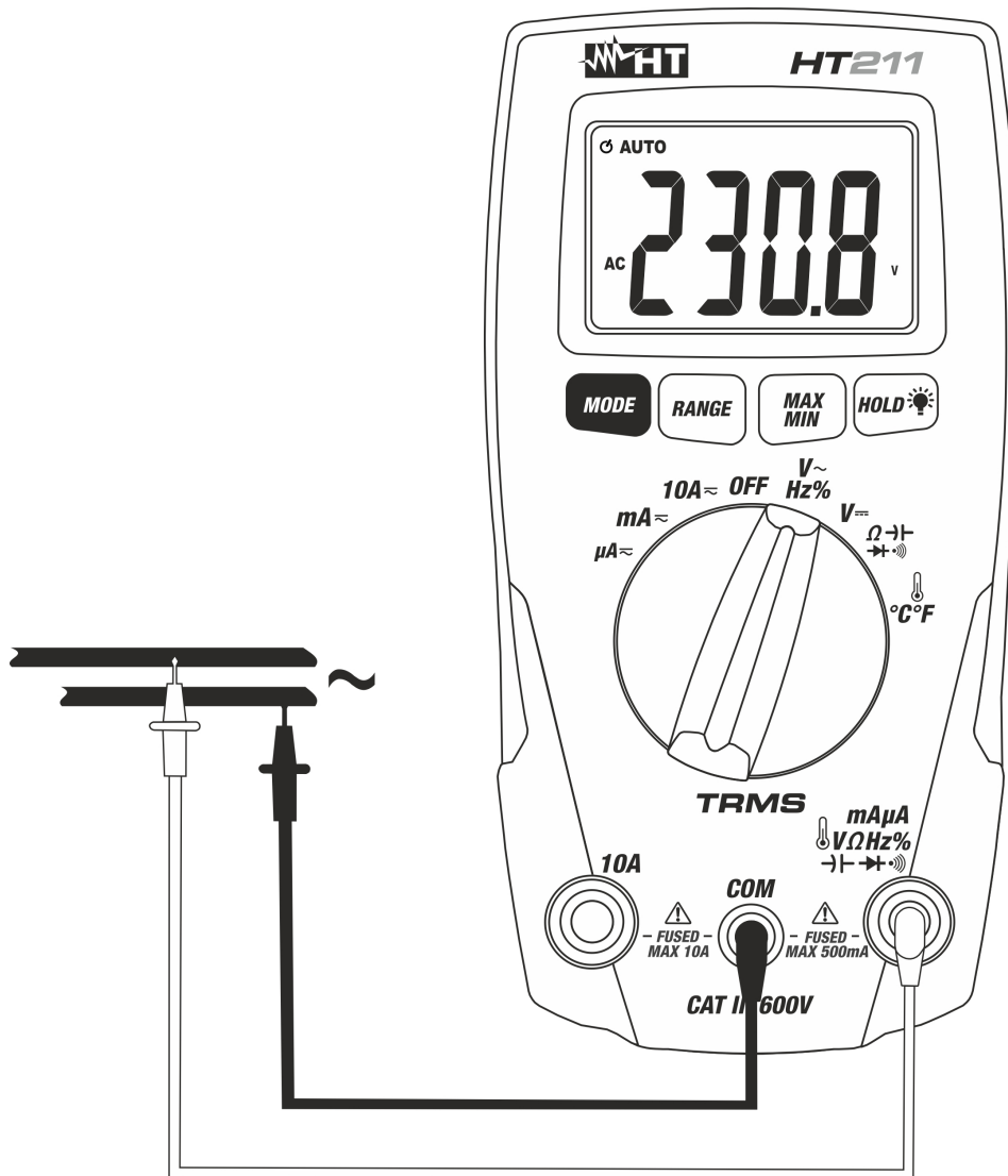
Fig. 3: Using the instrument for AC Voltage measurement
