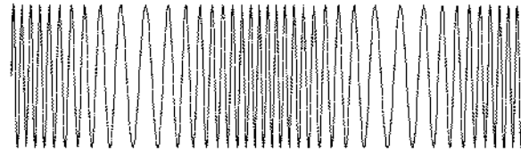
SIGNAL FROM PHASE MODULATOR
