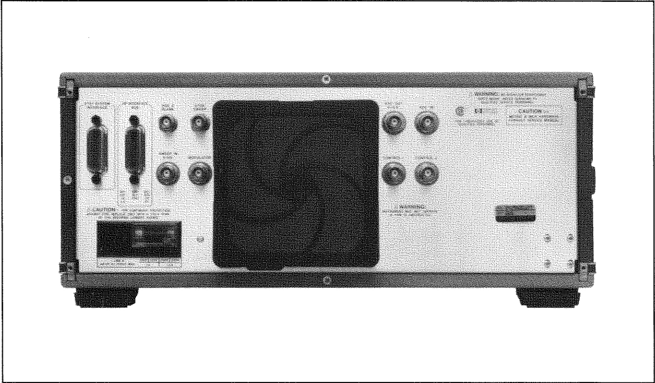
Figure 32. HP 8757A Rear Panel Connections
