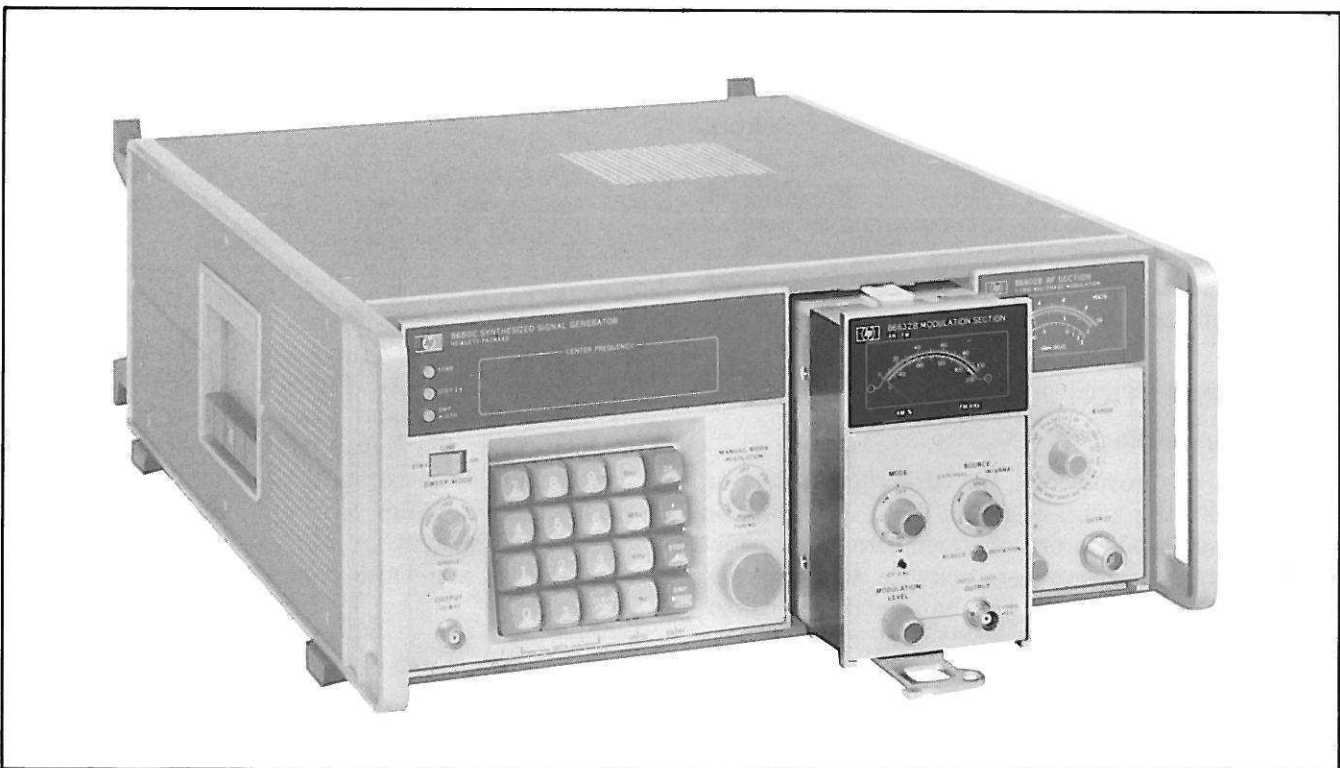
Figure 2-1. Model 86632B Being Installed in Mainframe
