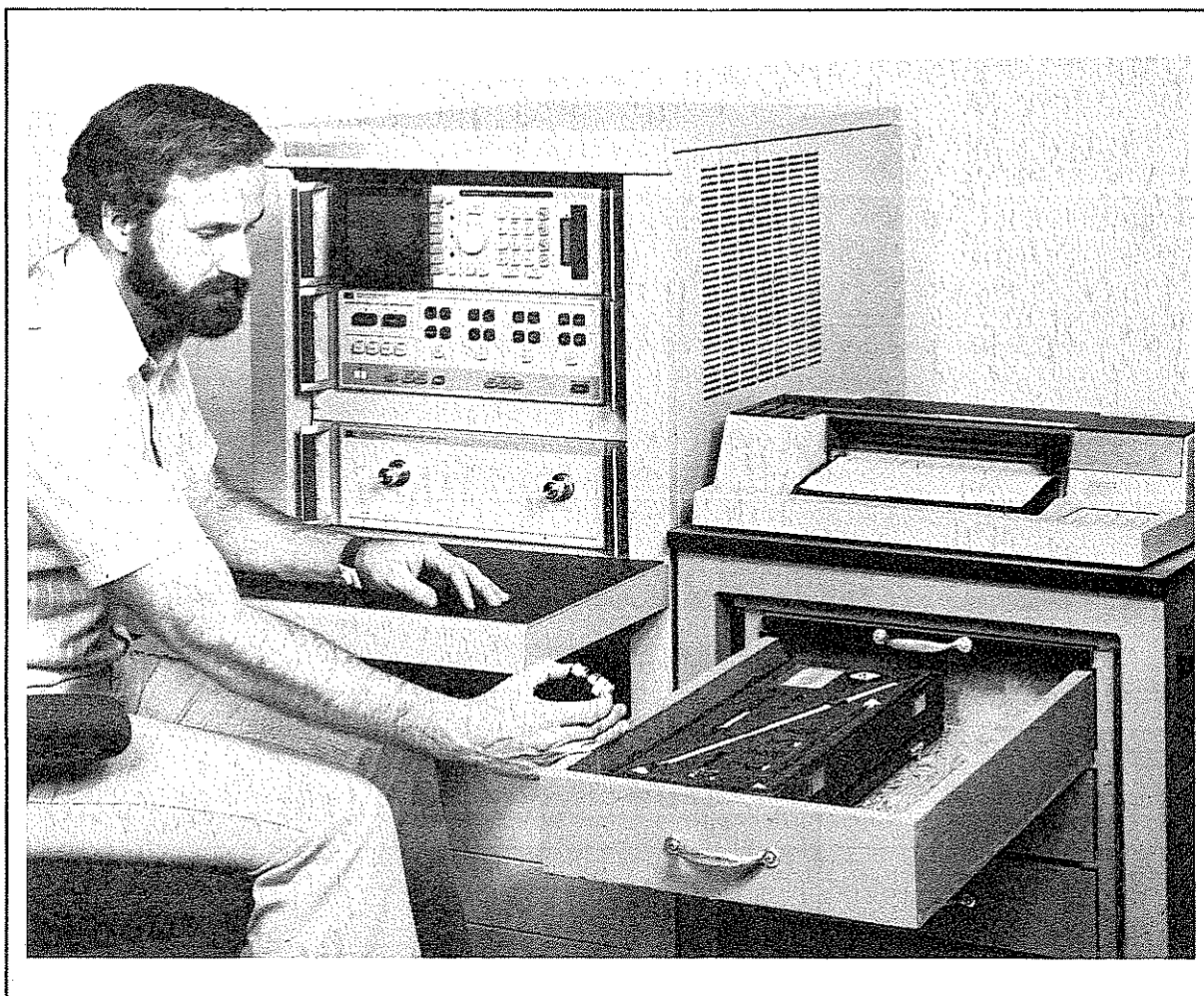
Figure 3. Calibration Kit Storage, Cover Removed
