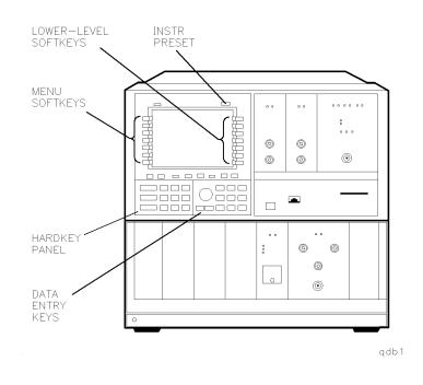
The HP 71209A modular spectrum analyzer has a full-band sweep from 100 Hz to 26.5 GHz and built-in external millimeter mixer capability. The standard system consists of an HP 70909A RF section, the HP 70004A color display, the HP 70001A mainframe, the HP 70900B local oscillator module, the HP 70902A and HP 70903A IF sections, and an HP 70310A precision frequency reference. Options on the standard system can add or delete modules.
