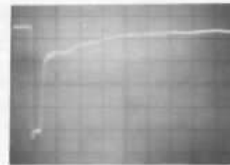
8 IC3(8). Normal operation. H = 0.1 \mu\text{sec}/\text{div} , V = 1V/div.
