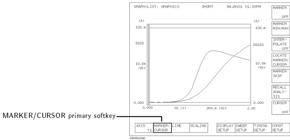
2. Select **MARKER** secondary softkey so that **ON** appears on the softkey. The **MARKER** softkey is highlighted, and the markers appears on the measurement curve.
