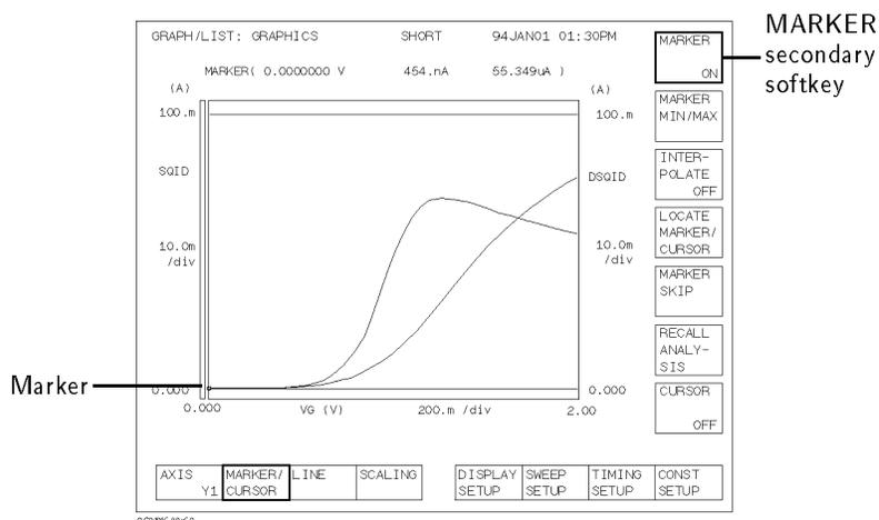
3. Select **AXIS** primary softkey so that **Y2** appears on the softkey. The **Y2** axis is highlighted.
