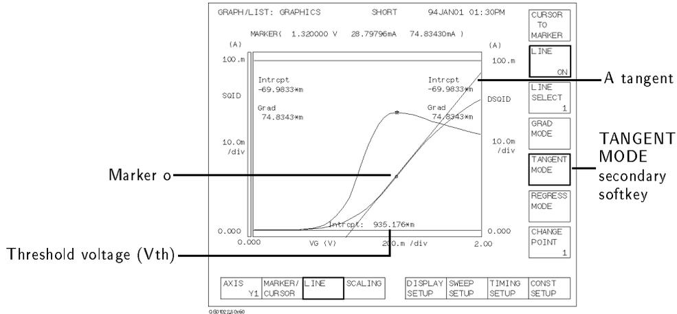
Read the X-axis intercept value of the tangent line. This is the threshold voltage ( $V_{th}$ ). In the example above,  $V_{th}$  is 935 mV.
