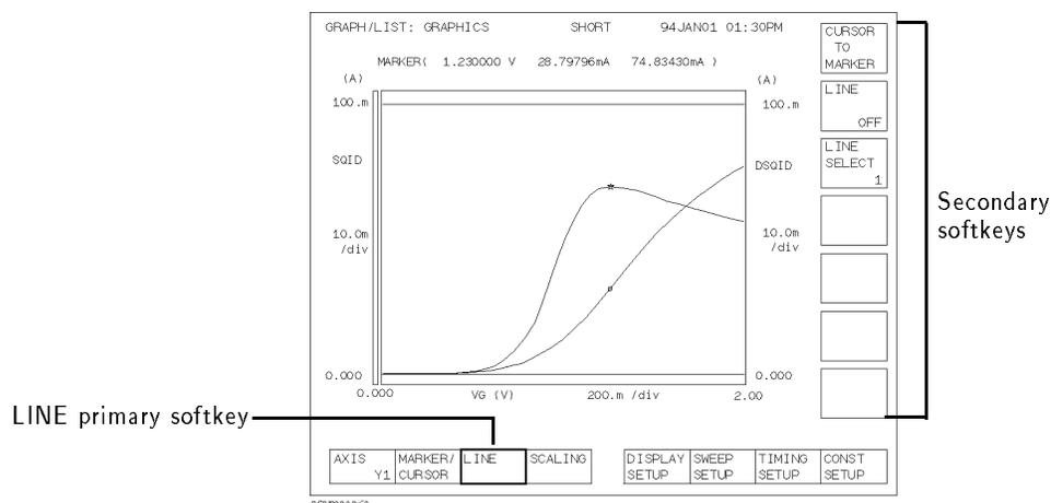
7. Select **LINE** secondary softkey so that **ON** appears on the softkey. The **LINE** softkey is highlighted, and a vertical line appears in the center of the plotting area.
