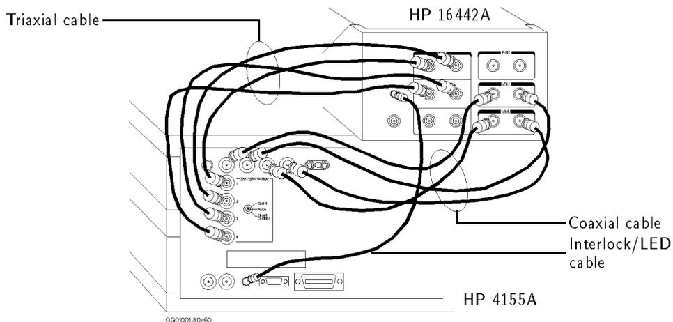
Connecting HP 4155A to HP 16442A Test Fixture
