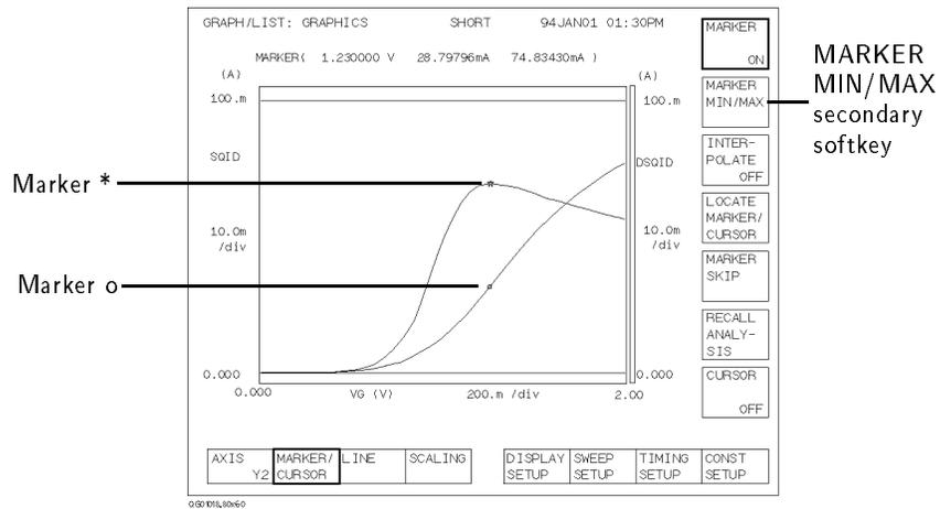
5. Select **AXIS** primary softkey so that Y1 appears on the softkey. The Y1 axis is highlighted.
