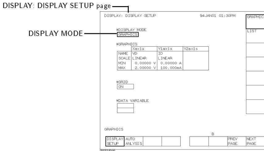
2. Make sure **GRAPHICS** is displayed in the DISPLAY MODE field. If not, select **GRAPHIC** secondary softkey in the DISPLAY MODE field.
