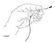
Figure 2-10. Connecting Grabbers to Test Points
