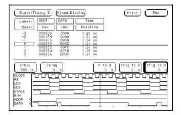
Figure 6-15. Timing/State Mixed Mode Display
