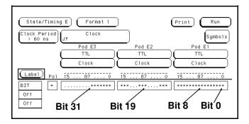
Figure 5-10. Numbering of Assigned Bits
