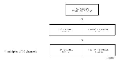
Figure 1-2. HP 16510B Configuration Capabilities
