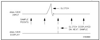
Figure 5-34. Glitch in Timing Waveform
