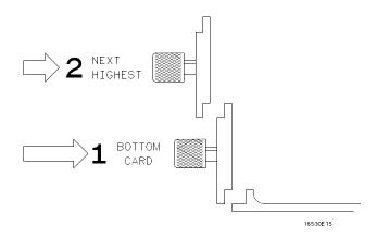
Figure A-3. Endplate Overlap (Installing)
