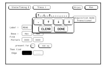
Figure 5-44. Combination of Edges Specified
