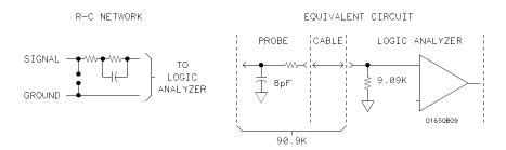
Figure 2-5. Probe Input Circuit
