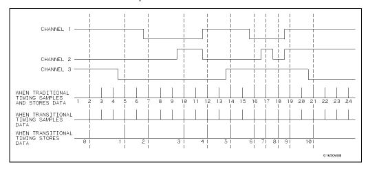
Figure 5-32. Transitional Timing vs. Traditional Timing
