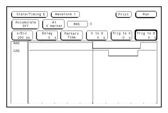
Figure 7-9. Waveform at 200 ns/Div
