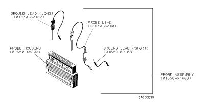
Figure 2-3. Probe Assembly
