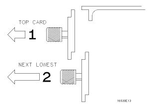
Figure A-1. Endplate Overlap (Removing)
