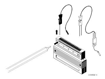
Figure 2-8. Disconnecting Probes from Pods
