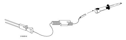
Figure 2-9. Connecting Grabbers to Probes
