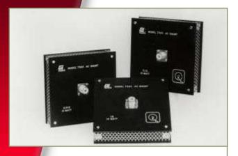
uildline 7320 series of four terminal AC Current Shunts feature low uncertainty (high accuracy), low temperature coefficients, and excellent stability. The shunts are designed to be purely resistive with extremely small values of reactance. The shunts may be used over a wide frequency range from DC to 100 kHz.
