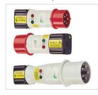
The A3-16, A3-32 and A3-63 three-phase current adapters are used for the convenient connection of test instruments to 5-pole CEE outlets. The three different versions have different sized plugs which correspond to 5-pole CEE outlets with current ratings of 16 A, 32 A and 63 A. Phase sequence is indicated with lamps.
