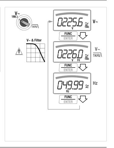
5.1.3 Alternating Voltage and Frequency Measurement V AC and Hz with Selectable Low-Pass Filter (METRAHIT EXTRA, METRAHIT ETECH and METRAHIT ESPECIAL only)
