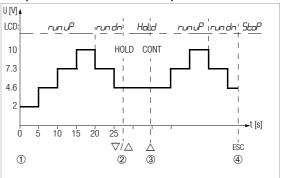
**Interval parameters:** output quantity: U (range of  $0 \dots 15$  V), SER-L = 2 V, End = 10 V, number of interval SEEP5 = 3, L = 5 s, RadE = RuLa
