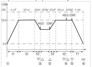
**Ramp parameters:** output quantity: U (range of 0 ... 15 V),  $5 \pm Rr \pm 2 = 2$  V, Erd = 10 V, E = 5 s, E = 8 s, E = 5 s, E = 6 s, E
